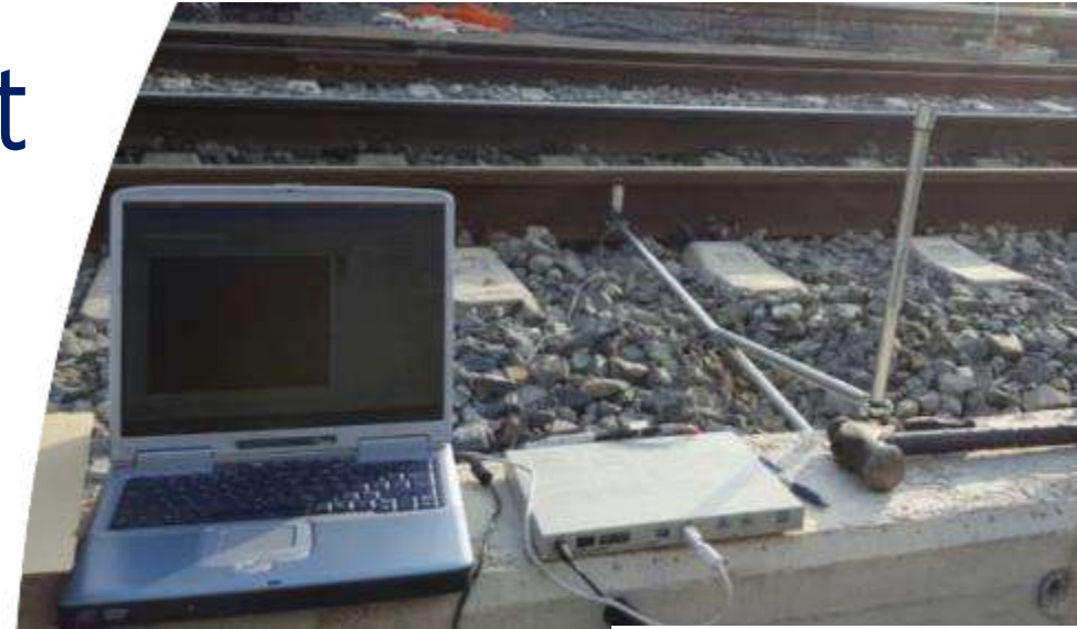
3GSM/3G enabled, GPS device based on ATmega328 (Arduino)
